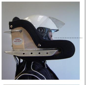
Mount shoulder restraints, using 2 bolts on each leave slightly loose to allow adjustment. Make sure large washers are used on slots. Get driver to sit in seat with arms as they would with hands on steering wheel in car. Adjust shoulder restraints to be firm against drivers shoulders. When in position tighten bolts.
