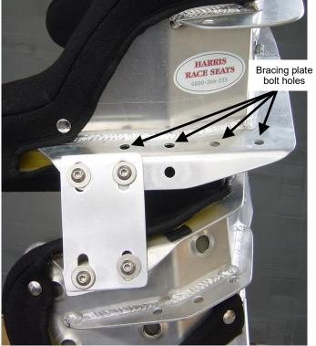
Head restraint must be braced to the roll cage to give maximum support. Use two mounting holes (shown in photo) to bolt your plates onto. You will need 5/16" (8mm) bolts and lock nuts.
