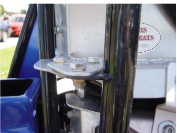
Weld tags to roll cage. Bolt brace plates onto Head restraint and roll cage tags with 5/16" (8mm) bolts.
