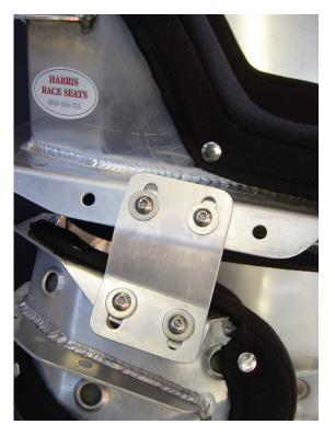
Once the Head and Shoulder restraints have been adjusted and all bolts tightened you need to fit slotted joiner plates as per photos. You may need to bend/fold these plates to suit.
